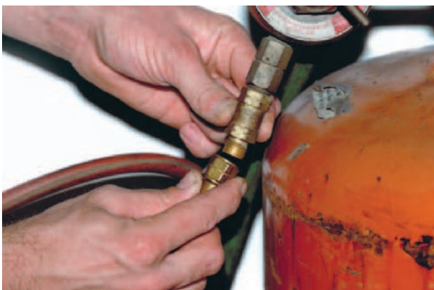
FIGURE 3-50 Attach reverse flow valves. Courtesy of Larry Jeffus.
