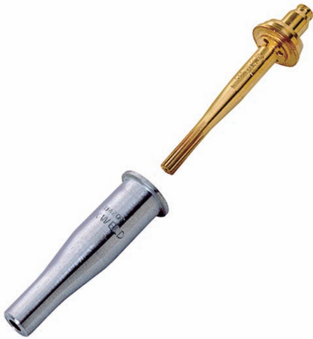
FIGURE 6-11 Tap the back of the torch head to remove a tip that is stuck. The tip itself should never be tapped.
