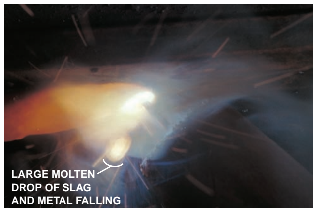
FIGURE 14-44 Hold the gun so that weld spatter will not fall onto the gun. Courtesy of Larry Jeffus.
