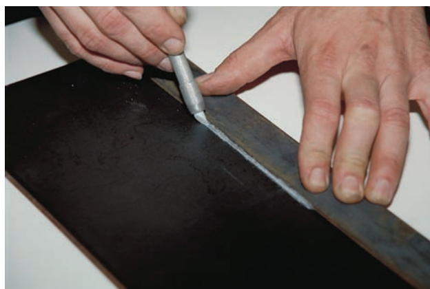
FIGURE 17-59 Be sure that the soapstone is held tightly to the part being traced. Courtesy of Larry Jeffus.
