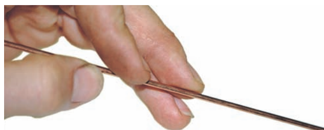
FIGURE 4-10 Feed the filler rod by using your index finger. Courtesy of Larry Jeffus.
