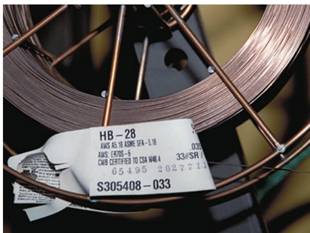
FIGURE 12-5 When installing the spool of wire, check the label to be sure that the wire is the correct type and size.
