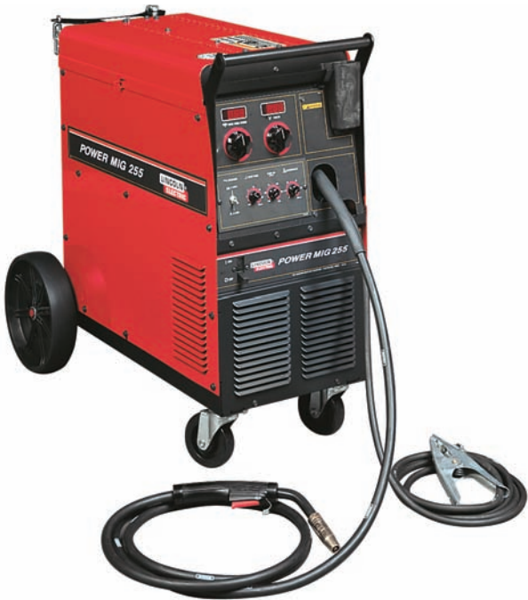
FIGURE 11-2 Semiautomatic GMA welding setup. Courtesy of Lincoln Electric Company.
