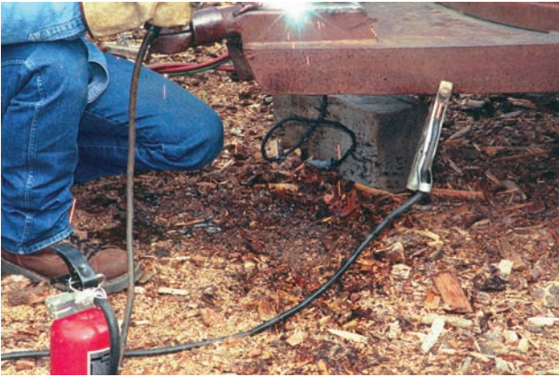
FIGURE 8-35 Make sure you have a good ground connection close to your welding. Courtesy of Larry Jeffus.
