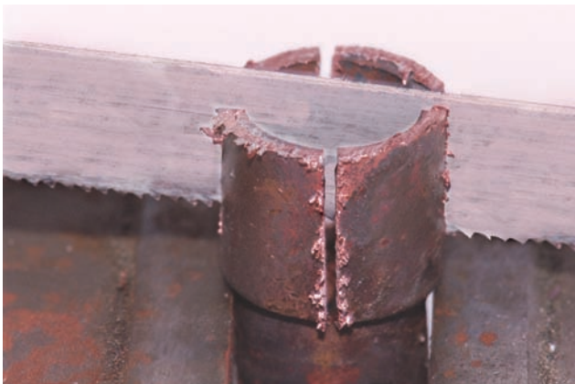
FIGURE 5-47 Quarter-saw the joint. Courtesy of Larry Jeffus.
