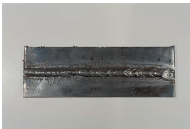
FIGURE 9-33 Stringer bead. Courtesy of Larry Jeffus.
