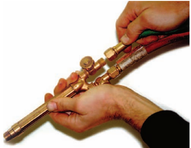
FIGURE 3-51 Connect the free ends of the oxygen (green) and the acetylene (red) hoses to the welding torch. Courtesy of Larry Jeffus.
