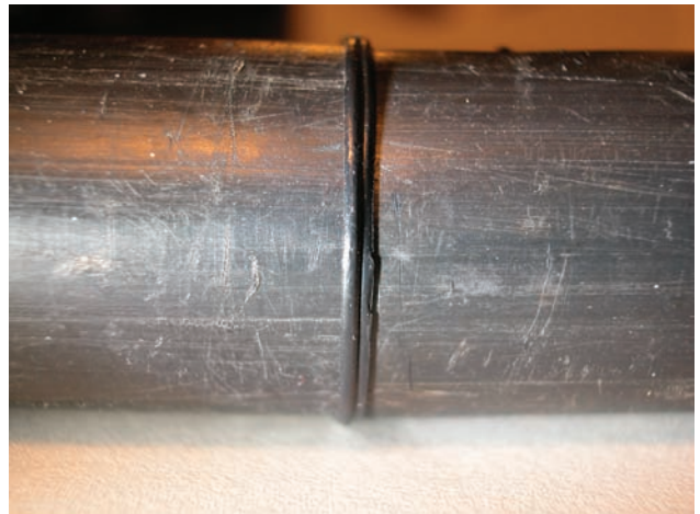
FIGURE 18-29 ABS butt weld. Courtesy of Larry Jeffus.
