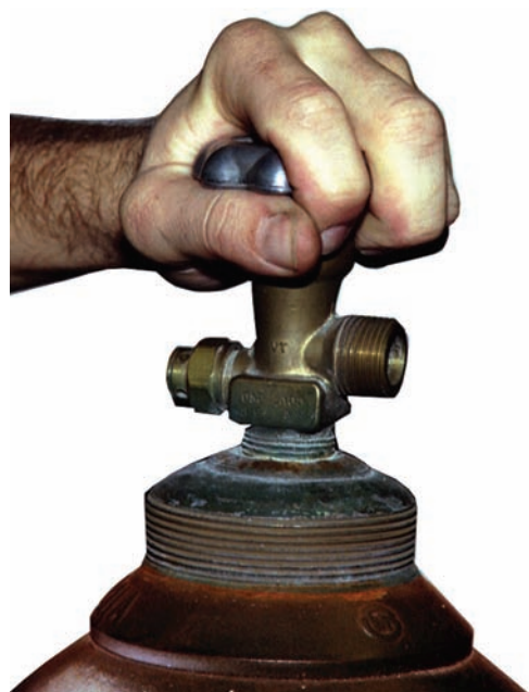
FIGURE 12-4 Blowing out dirt from the cylinder valve.
