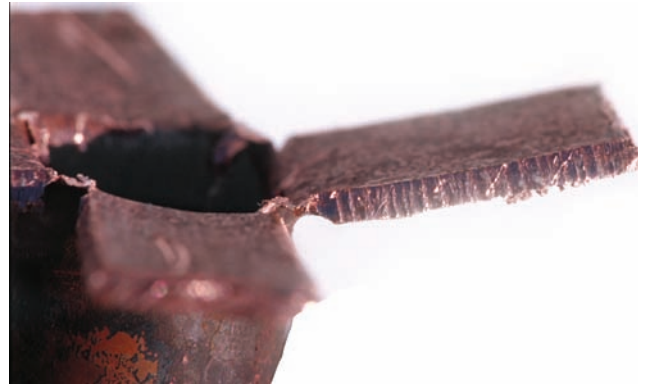
FIGURE 5-49 Complete joint fill. Courtesy of Larry Jeffus.
