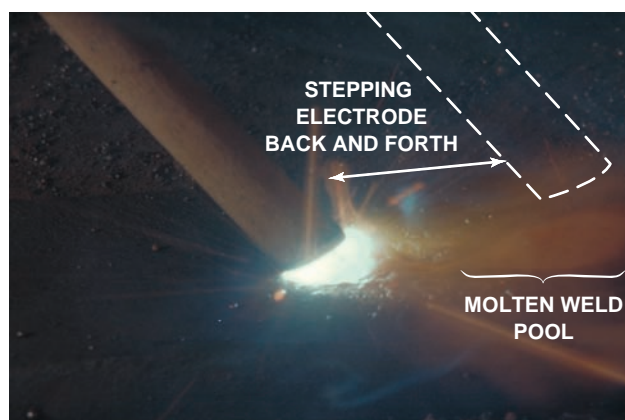
FIGURE 9-28 The electrode is moved slightly forward and then returned to the weld pool. Courtesy of Larry Jeffus.
