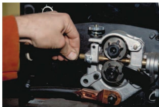
FIGURE 12-15 Push the wire through the guides by hand. Courtesy of Larry Jeffus.
