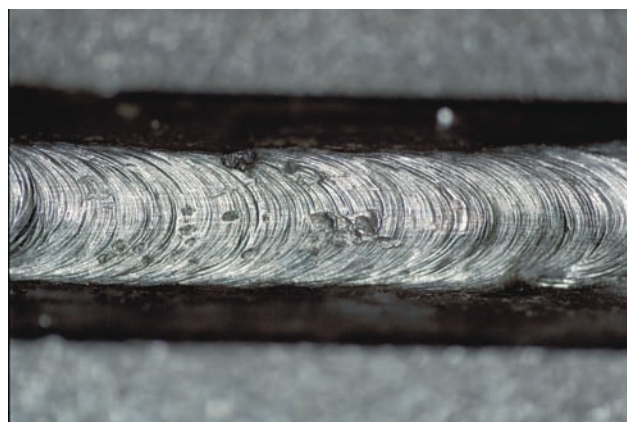
FIGURE 12-44 Weld bead made with GMAW pulsed arc metal transfer mode. Courtesy of Larry Jeffus.
