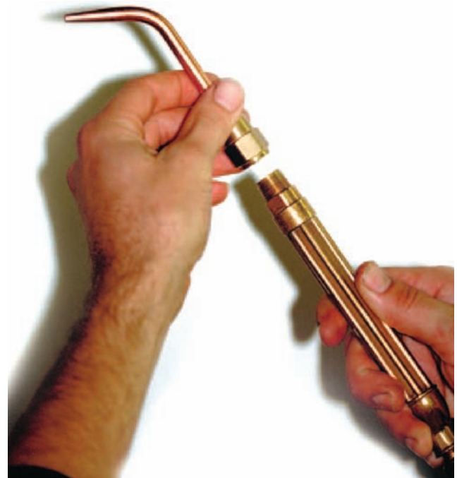
FIGURE 3-52 Select the proper tip or nozzle and install it on the torch body. Courtesy of Larry Jeffus.
