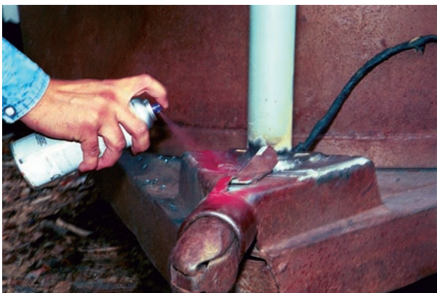
FIGURE 17-76 Spray paint the finished weld to keep it from rusting. Courtesy of Larry Jeffus.
