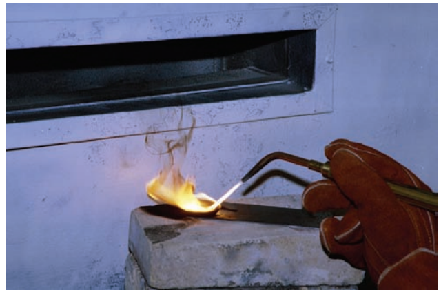
FIGURE 2-17 An exhaust pickup. Courtesy of Larry Jeffus.
