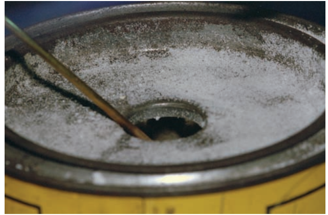
FIGURE 5-22(B) Dipping the heated rod into the flux. Courtesy of Larry Jeffus.
