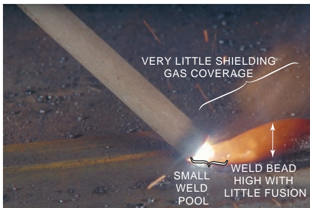
FIGURE 9-6 Welding with the amperage set too low.
