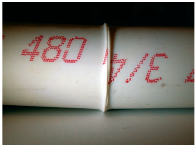
FIGURE 18-30 PVC butt weld. Courtesy of Larry Jeffus.
