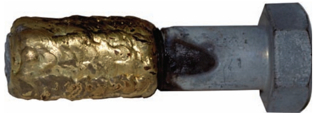
FIGURE 5-42 Round shaft built up with braze. Courtesy of Larry Jeffus.
