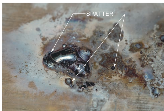
FIGURE 9-8 Hard weld spatter fused to base metal.
