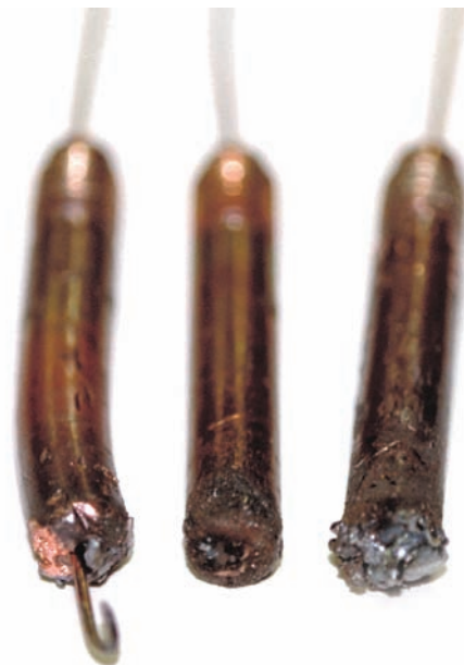
FIGURE 12-11 The contact tube must be the correct size. (A) Too small a contact tube will cause the wire to stick. (B) Too large a contact tube can cause arcing to occur between the wire and tube. (C) Heat from the arcing can damage the tube. (B) Courtesy of Brett V. Hahn. (C) Courtesy of Larry Jeffus.
