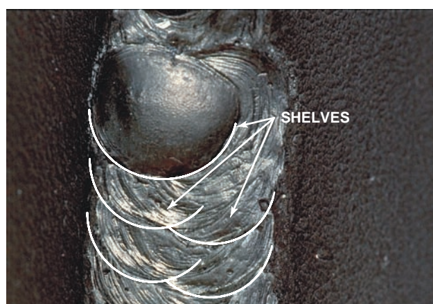
FIGURE 9-30 Using the shelf to support the molten pool for vertical welds. Courtesy of Larry Jeffus.
