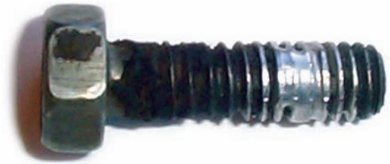
FIGURE 5-1(B) Solder has been applied to the threads to act as a lock tight. Courtesy of Larry Jeffus.
