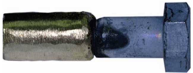
FIGURE 5-43 Shaft turned down to check for slag inclusions or poor bonding. Courtesy of Larry Jeffus.
