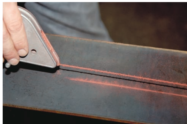
FIGURE 17-44(B) Check to see that the line is dark enough. Courtesy of Larry Jeffus.
