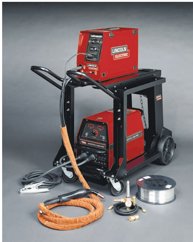
FIGURE 11-24 Wire-feed system that enables the wire to be moved through a longer cable. Courtesy of Lincoln Electric Company.
