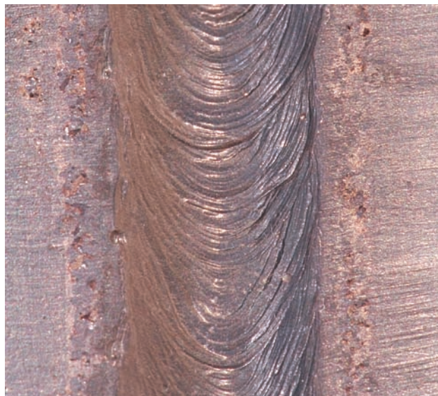
FIGURE 10-16 The root face must be uniform. Courtesy of Larry Jeffus.
